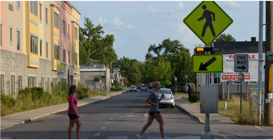
Figure 6-33. A Rectangular Rapid Flashing Beacon (RRFB)
