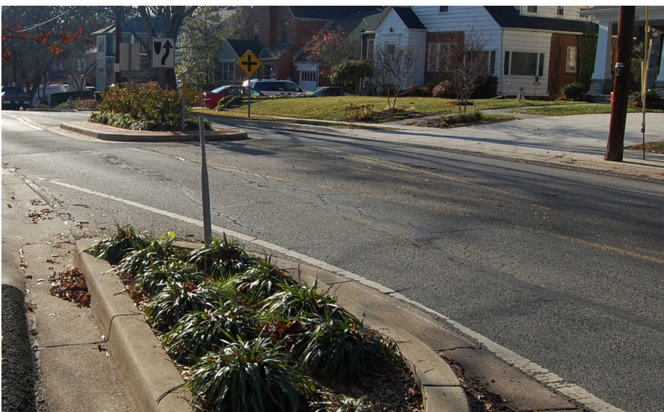
Figure 8-8. Horizontal traffic calming treatment
