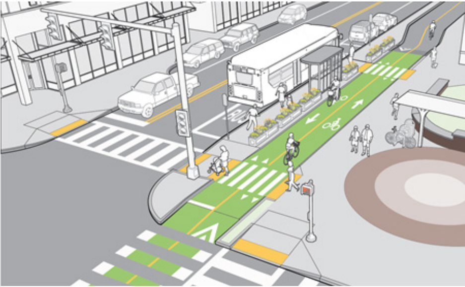
Figure 6-25. Bus boarding island (Note: This graphic shows an intermediate-level bikeway, which is the county's default. This creates a detectable edge between the sidewalk and the bikeway.)
