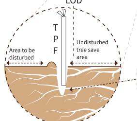
Root pruning shall be to the depth of excavation, or 24 inches, whichever is less.
