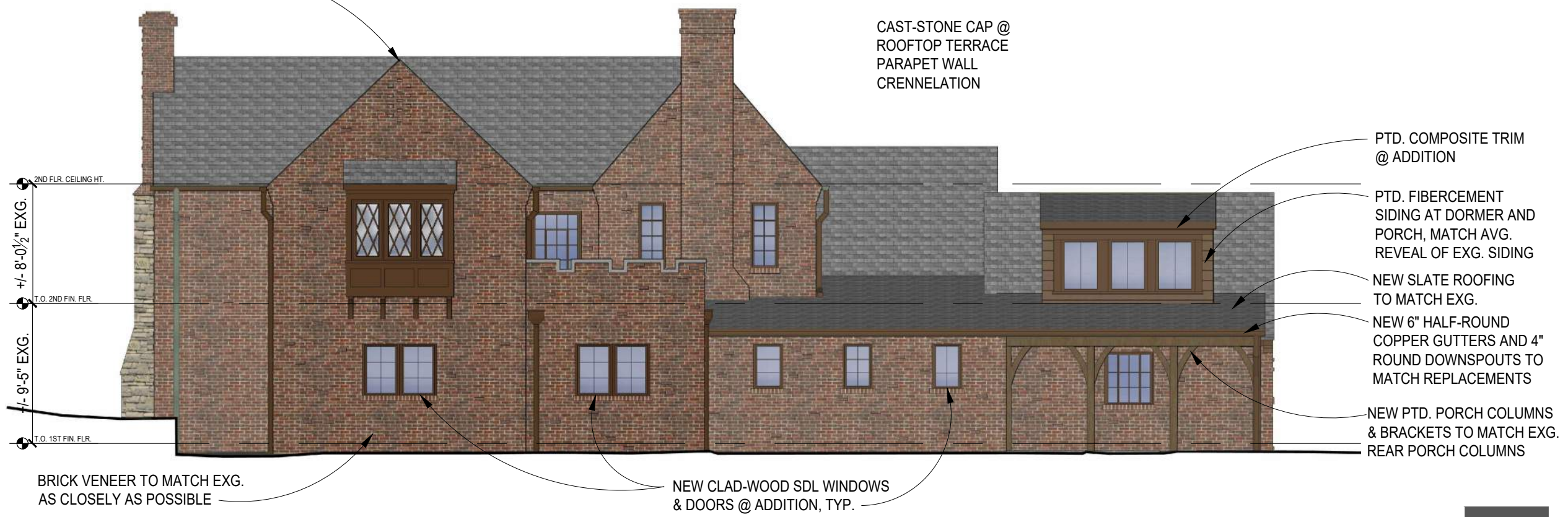
HOLD PEAK OF REAR ADDITION BELOW PEAK OF EXG. ROOF LINE EXISTING REAR ELEVATION
