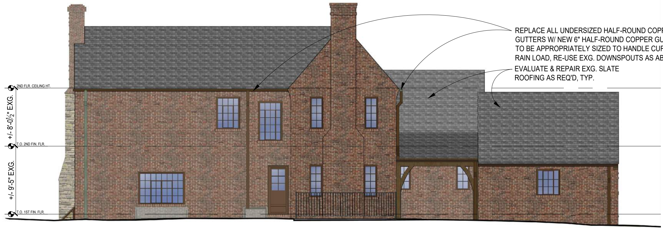
HOLD PEAK OF REAR ADDITION BELOW PEAK OF EXG. ROOF LINE EXISTING REAR ELEVATION
