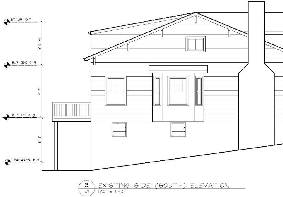
Figure 10: The existing left-side elevation. Note the elevation does not show the existing deck stairs.
