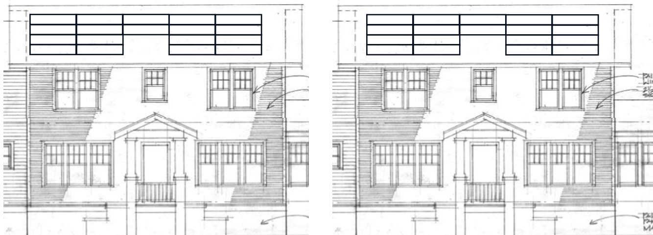
Figure 6: Proposed layout (slightly offset to the left), suggested recommended revision (centered on the roof). This small alteration would center the ‘gap’ symmetrically over the central window opening on the 2 nd floor. Note: dimensions of panels are approximate.
