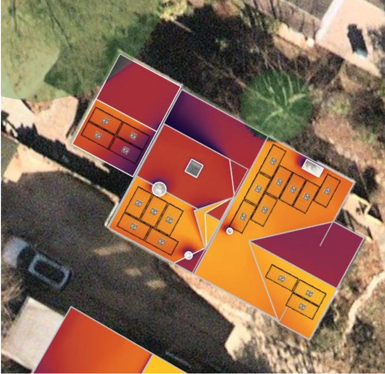
Figure 3: Roof heat map, showing the locations of the highest solar collection.
