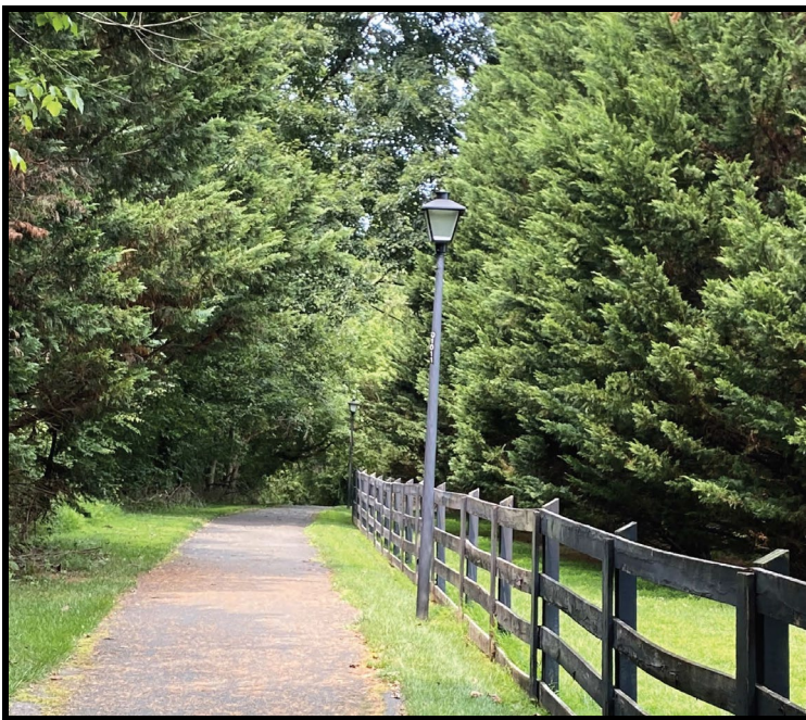
Figure 2: The applicant provided this representative photo of the proposed 12-foot tall fiberglass post with “Colonial” light at the top.
