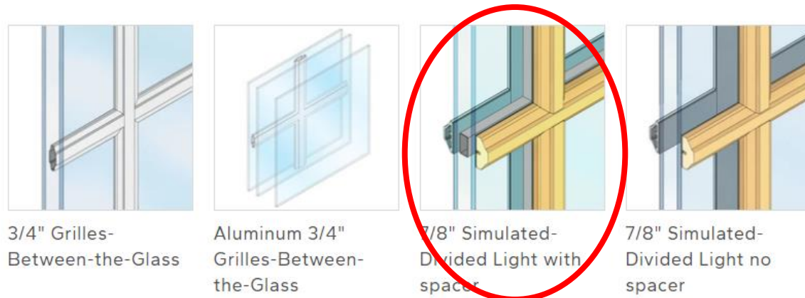
Figure 5: Grille profile options from Pella, Staff recommends the HPC require simulated divided light with spacer (circled) instead of the proposed grilles between the glass (far left).
