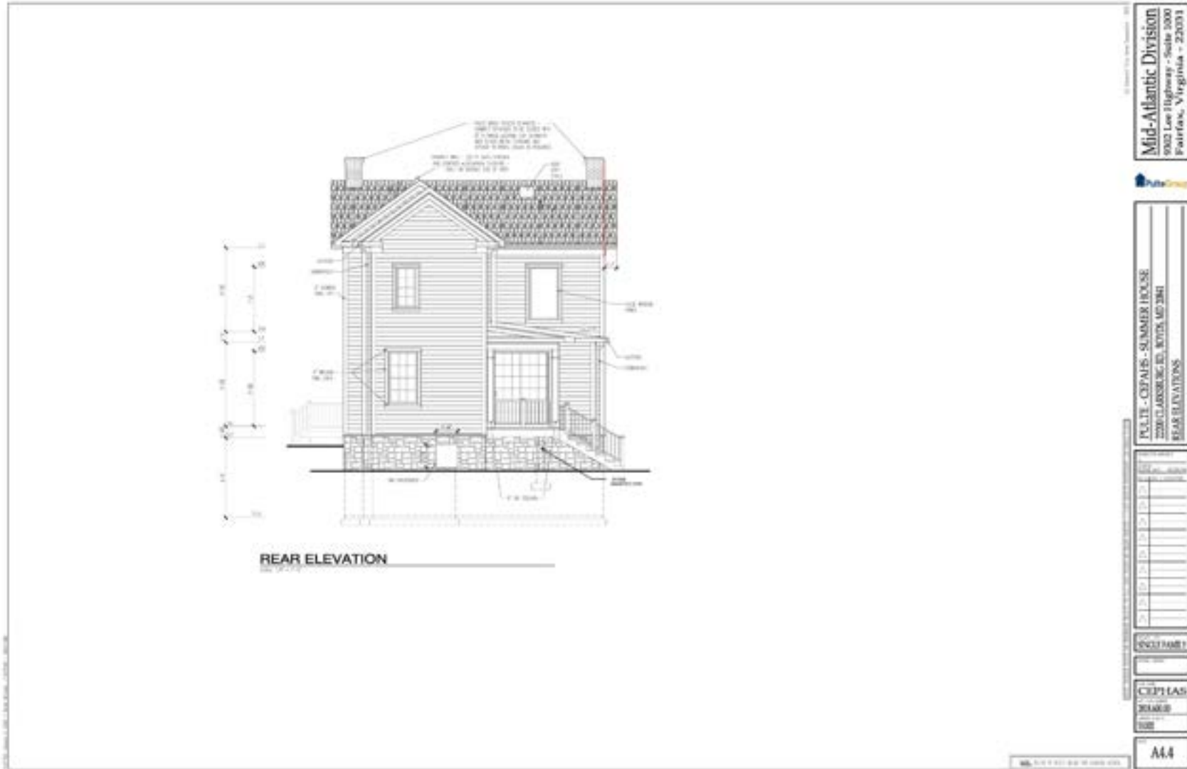
Figure 16: The rear elevation provided as part of this submission. Changes include regrading and the addition of gutters and downspouts; roof vents; porch railings, wrapped porch posts, and an HVAC condenser.
