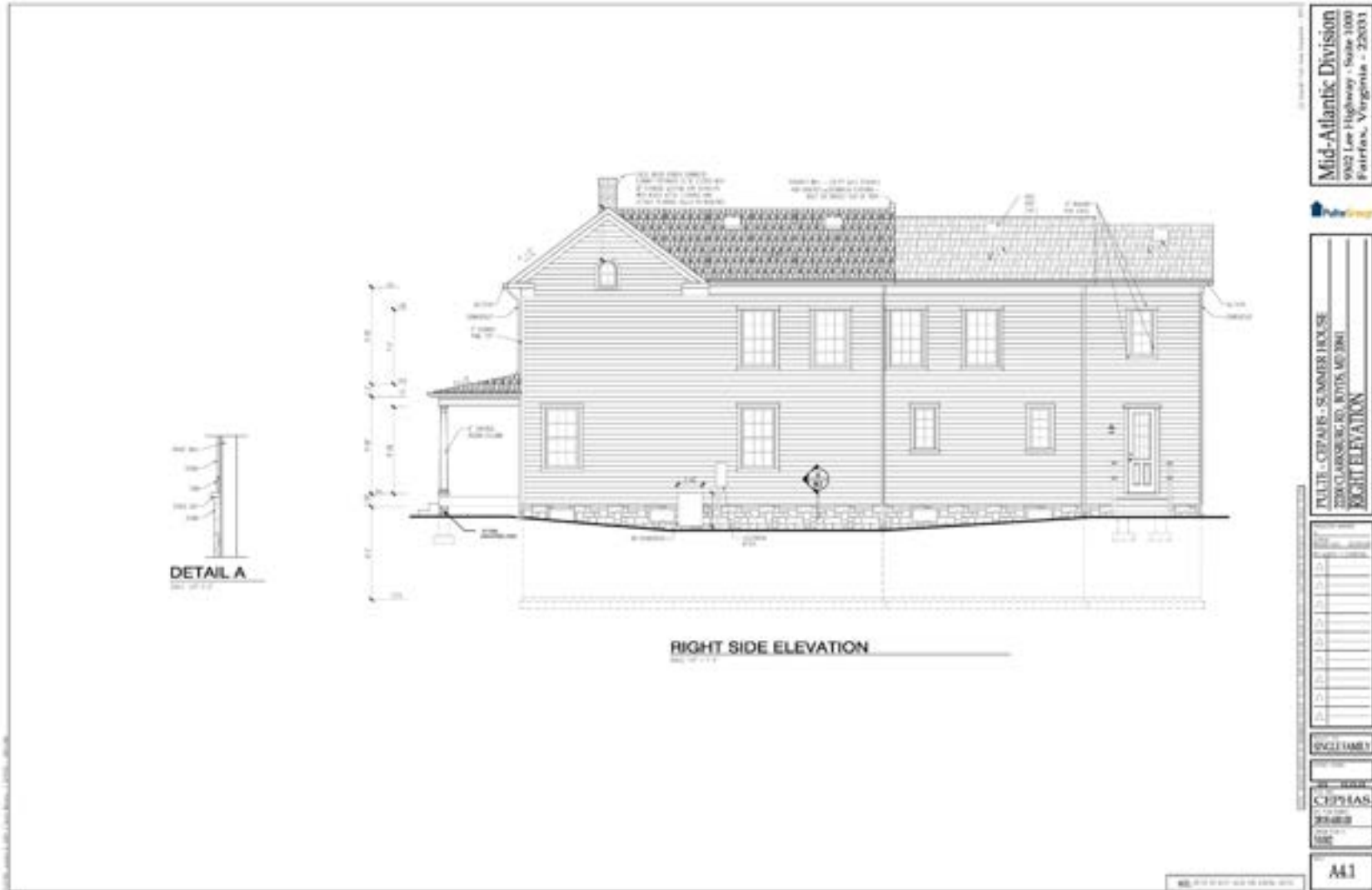
Figure 9: The right-side elevation provided as part of this submission. Changes include new grading and the addition of gutters and downspouts; wrapped porch posts, basement vinyl hopper windows, and an HVAC condenser.
