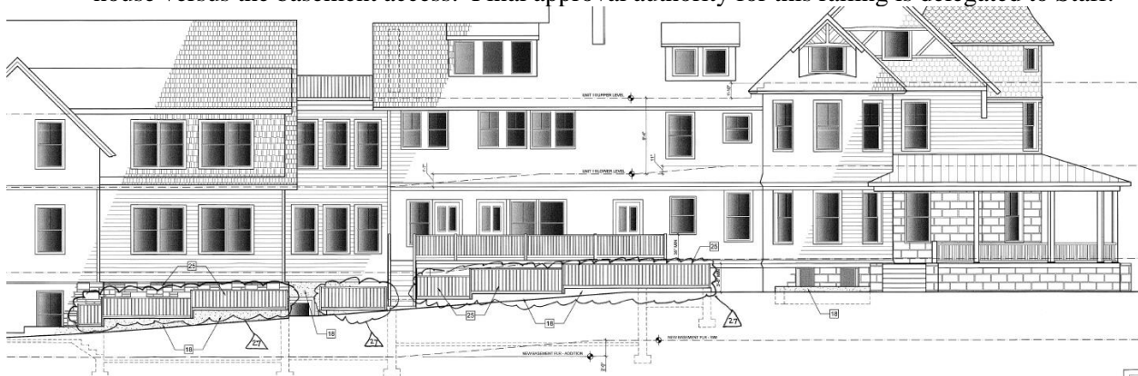
Figure 6: Proposed east elevation showing the railing for the patios and the railing for the 1st-floor side porch.
