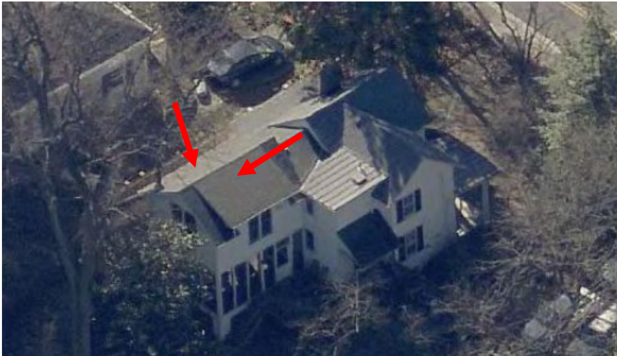
Figure 3: Aerial view showing the rear and side elevations of the subject house. The red arrows point to the locations of the two proposed arrays on the non-historic addition constructed in 2010. Source: ConnectExplorer.
