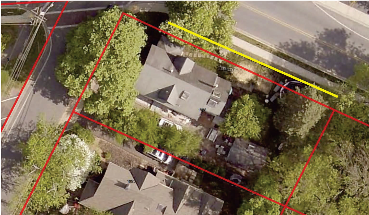
Figure 3: The existing stockade fence (highlighted in yellow) is outside the property boundary (shown in red).
