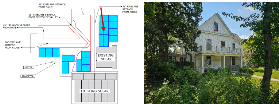
Figure 5: Roof plan showing the proposed solar array (left) and view of the facade from Columbia Avenue. The red arrow points to the proposed solar array visible from Columbia Avenue.
