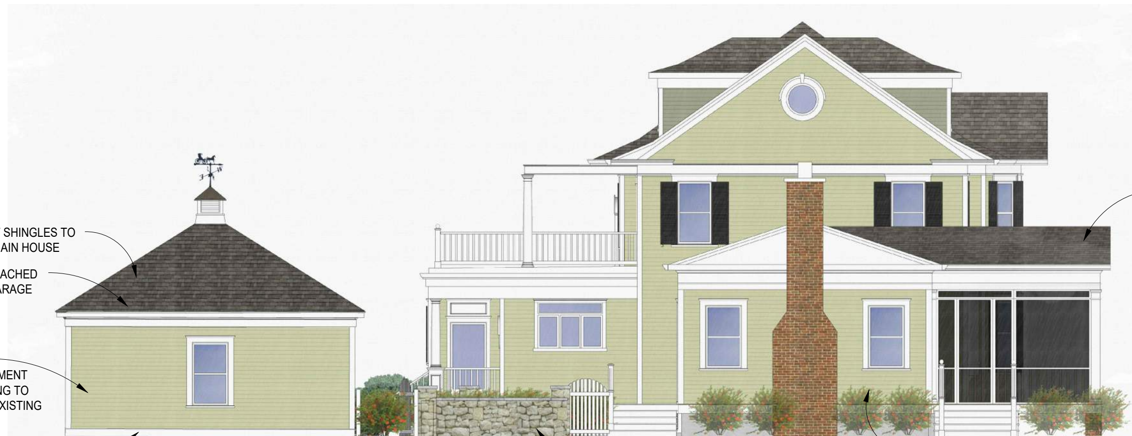
2 PROPOSED REAR ELEVATION SCALE: 1/8"=1'-0"
