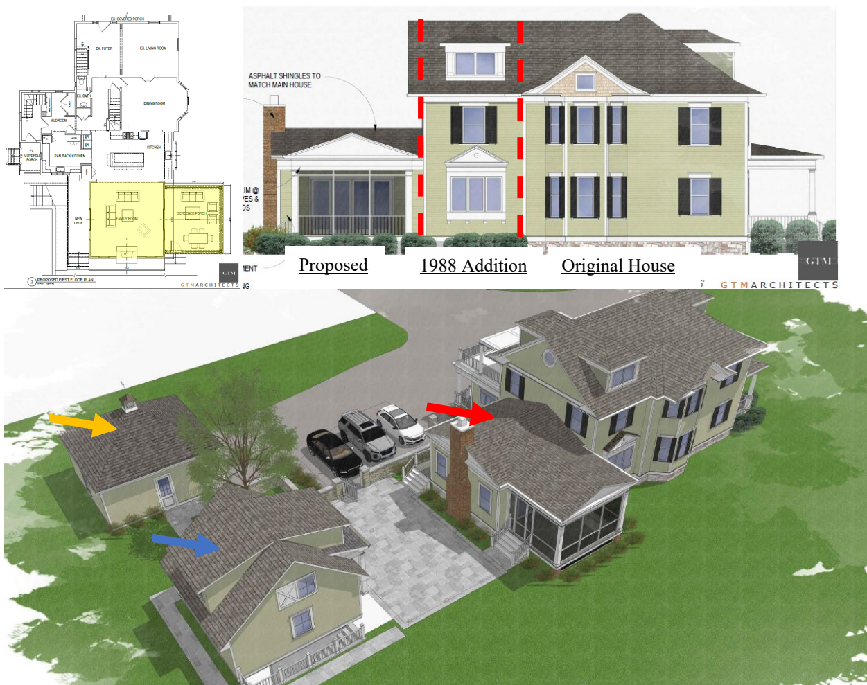
Figure 4: Floorplan (new additions are highlighted yellow), south elevation showing the evolution of the house, and oblique views of the proposal. The red arrow points to the addition, the yellow arrow to the proposed garage, and the blue arrow to the existing accessory dwelling unit.
