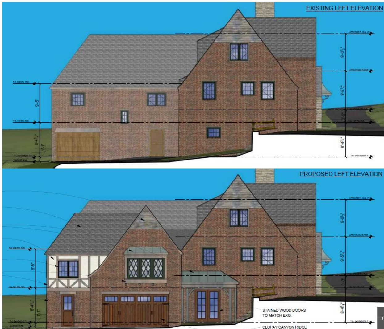
Figure 5: Existing left elevation (above) and proposed (below).
