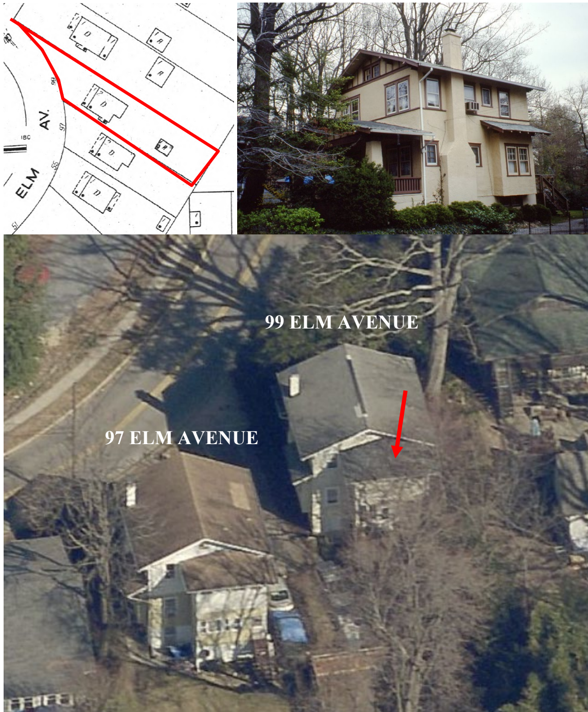
Figure 2: Sanborn Fire Insurance Map showing the current footprint of the house in 1927 (upper left), view of the north (façade) and west elevations ca. 1990 (upper right), and oblique aerial view of the rear elevation showing the enclosed two-story sleeping porch (red arrow) on the rear elevation of the subject house at 99 Elm Avenue. Note that the adjacent house at 97 Elm Avenue has a matching plan and fenestration pattern. Source: Sanborn Fire Insurance Map, Montgomery Planning, and Connect Explorer.
