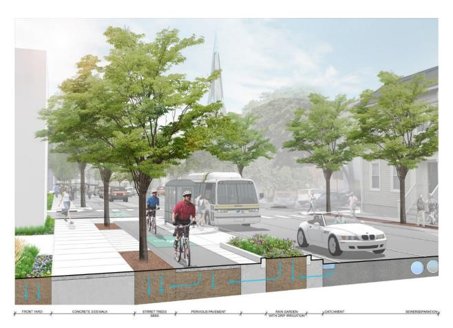
Exhibit: Rendering of potential stormwater treatment within the right-of-way
