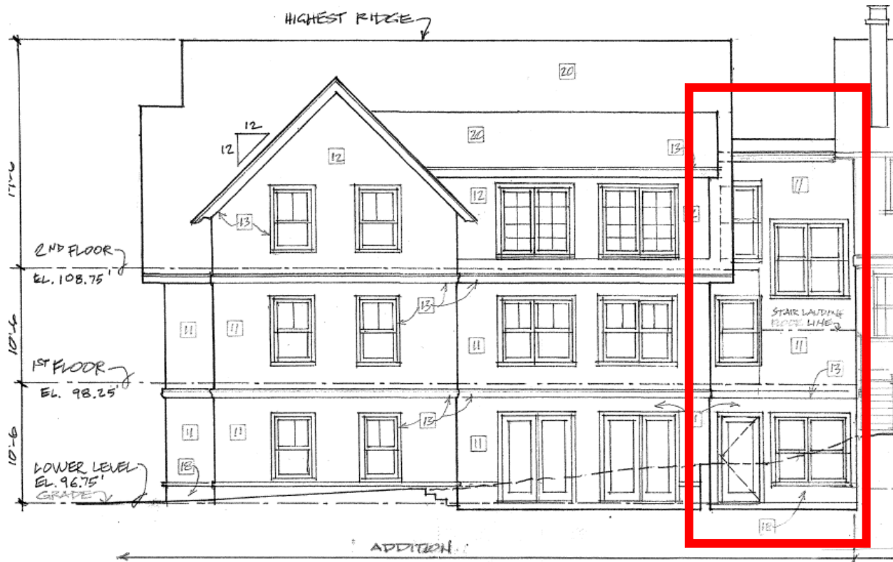
Figure 7: The east elevation of the proposed addition showing the revised hyphen design.
