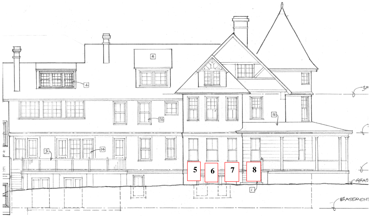
Figure 5: The east elevation with the historic windows to be retained labeled.
