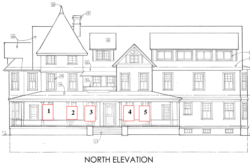
Figure 4: The north elevation with the retained historic windows labeled.
