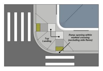
Perpendicular curb ramps directly aligned with appropriate crosswalks. Image Credit: U.S. Access Board
