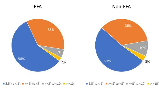
Street buffer width is the distance between the pathway and the curb. Street buffers separate moving vehicles from pedestrians, and they may allow the planting of larger street trees to provide robust physical separation from traffic, shade canopy, and a sense of enclosure for pedestrians. Without a buffer, pedestrians may "shy away" from adjacent travel lanes, effectively using part of the pathway as a buffer from the road, reducing the pathway's effective width.
