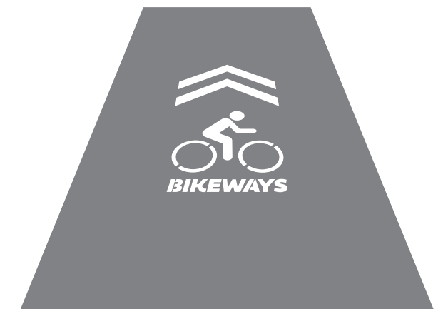
B4 Pavement Marking 2'-2" w x 4'-0" h
