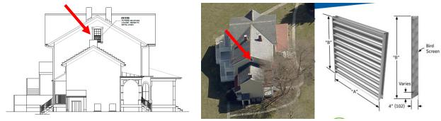
Figure 5: View of the west elevation showing the subject window (red arrows) and the proposed louvered intake vent to replace the lower-sash of the window. Source: Montgomery Parks, Connect Explorer, and Ruskin.
