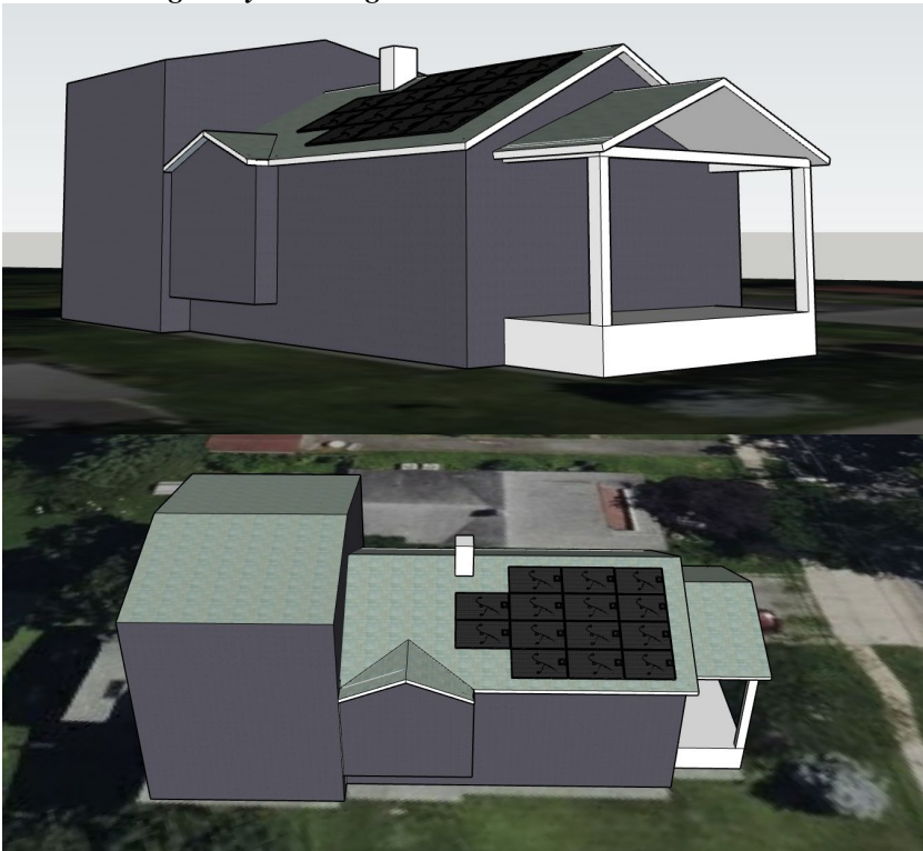
Figure 7: Illustrative model showing staff's recommended fourteen (14) panel array on the southern slope of the historic house. Note, the drawing does not include the solar arrays on the two-story addition. Source: Montgomery Planning.
