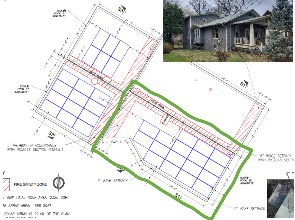
Figure 5: Solar panel layout submitted by the applicant. The green square shows the proposed location of the seventeen (17) panels on the southern slope of the historic house. Source: Solar Energy World.
