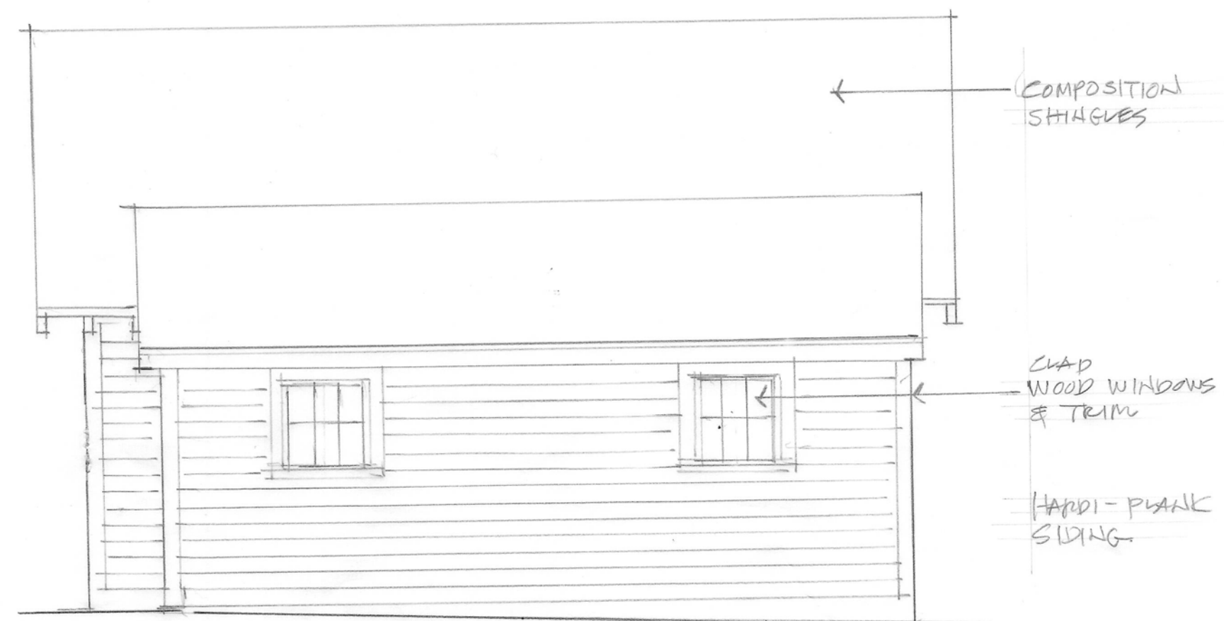
EXISTING RIGHT SIDE ELEVATION. Scale: 1/4" = 1'-0"
