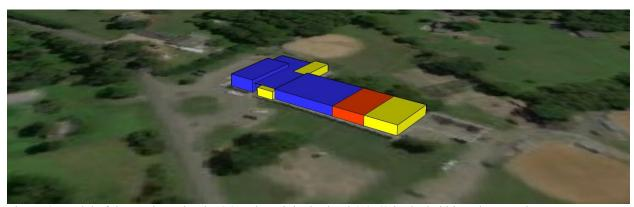
Figure 6: Model of the Taylor School, 1961. The original school (1952) is shaded blue, the two-classroom addition (1954) is shaded orange, and the extension of the principal's office near the main entrance, teacher's lounge and health room on the rear elevation, and two-classroom addition are shaded yellow (1961).
