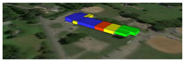
Figure 8: Model of the Taylor School, 1969. The original school (1952) is shaded blue. The two-classroom addition (1954) is shaded orange. The extension of the principal's office near the main entrance, teacher's lounge and health room on the rear elevation, and two-classroom addition are shaded yellow (1961). The library and services wing is shaded green (1969).
