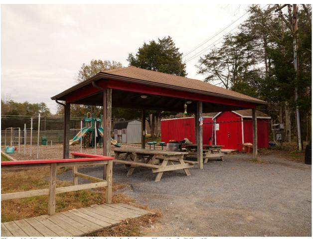
Figure 18: View of wood-frame, hipped-roof, picnic pavilion (Outbuilding H).
