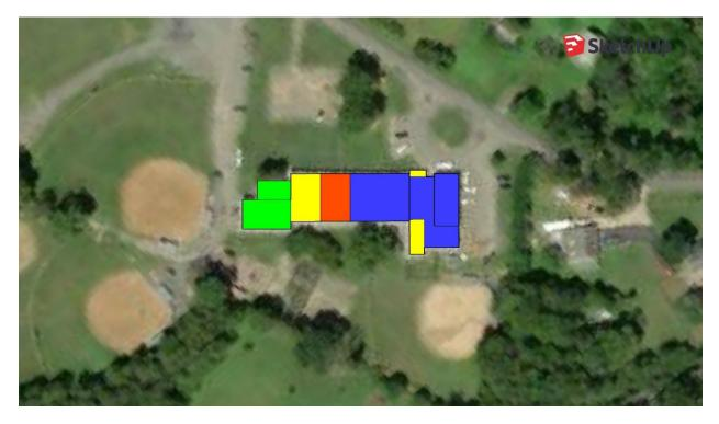
Figure 9: Model of the Taylor School, 1969. The original school (1952) is shaded blue. The two-classroom addition (1954) is shaded orange. The extension of the principal's office near the main entrance, teacher's lounge and health room on the rear elevation, and two-classroom addition are shaded yellow (1961). The library and services wing is shaded green (1969).
