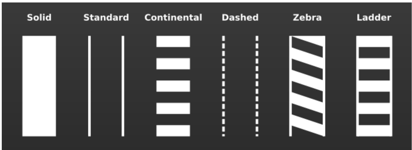
Figure 20. Standard High-Visibility Crosswalk Markings ( www.pedbikeimages.org/Charles Zegeer )
