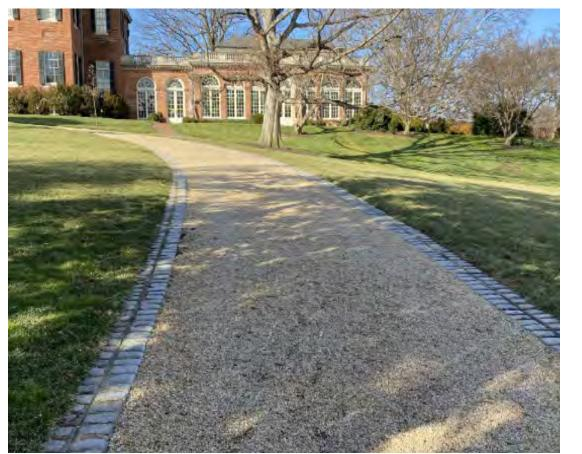
Design precedent of seeded aggregate concrete drive with cobble edge band.
