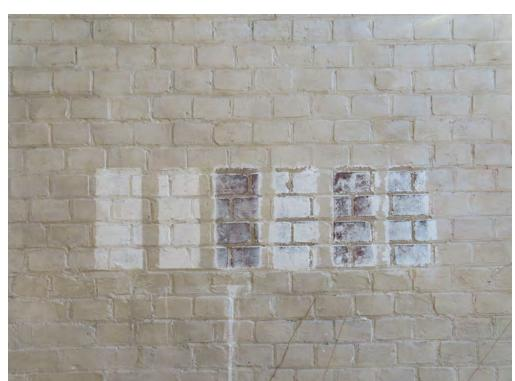
Paint Removal Cleaning Tests – Back to Nature Multi-Strip was the most successful stripper (red box).
