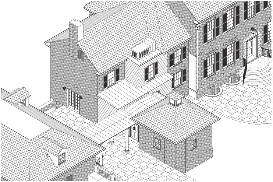
Bird's eye view of mechanical equipment located on flat seam metal roof of rear addition.
