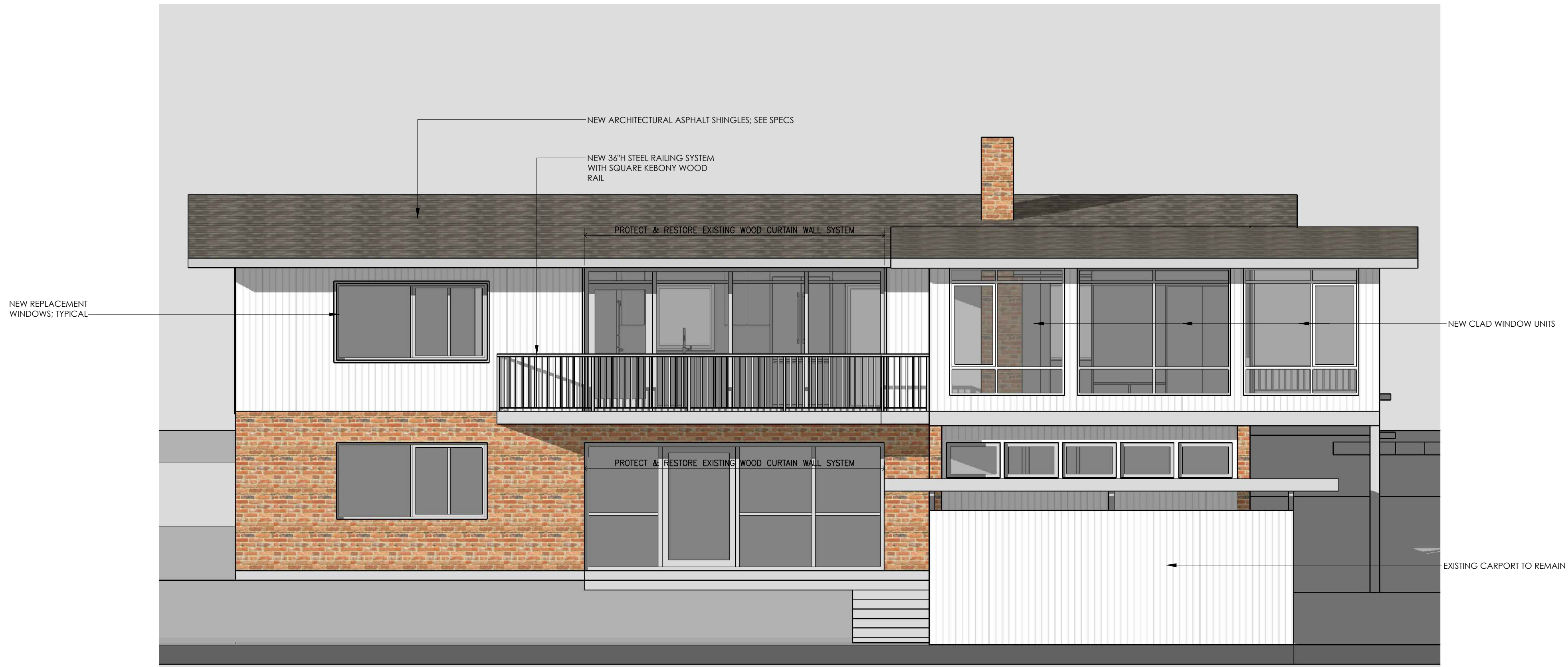
1 A200 1/4"=1'-0" PROPOSED FRONT ELEVATION
