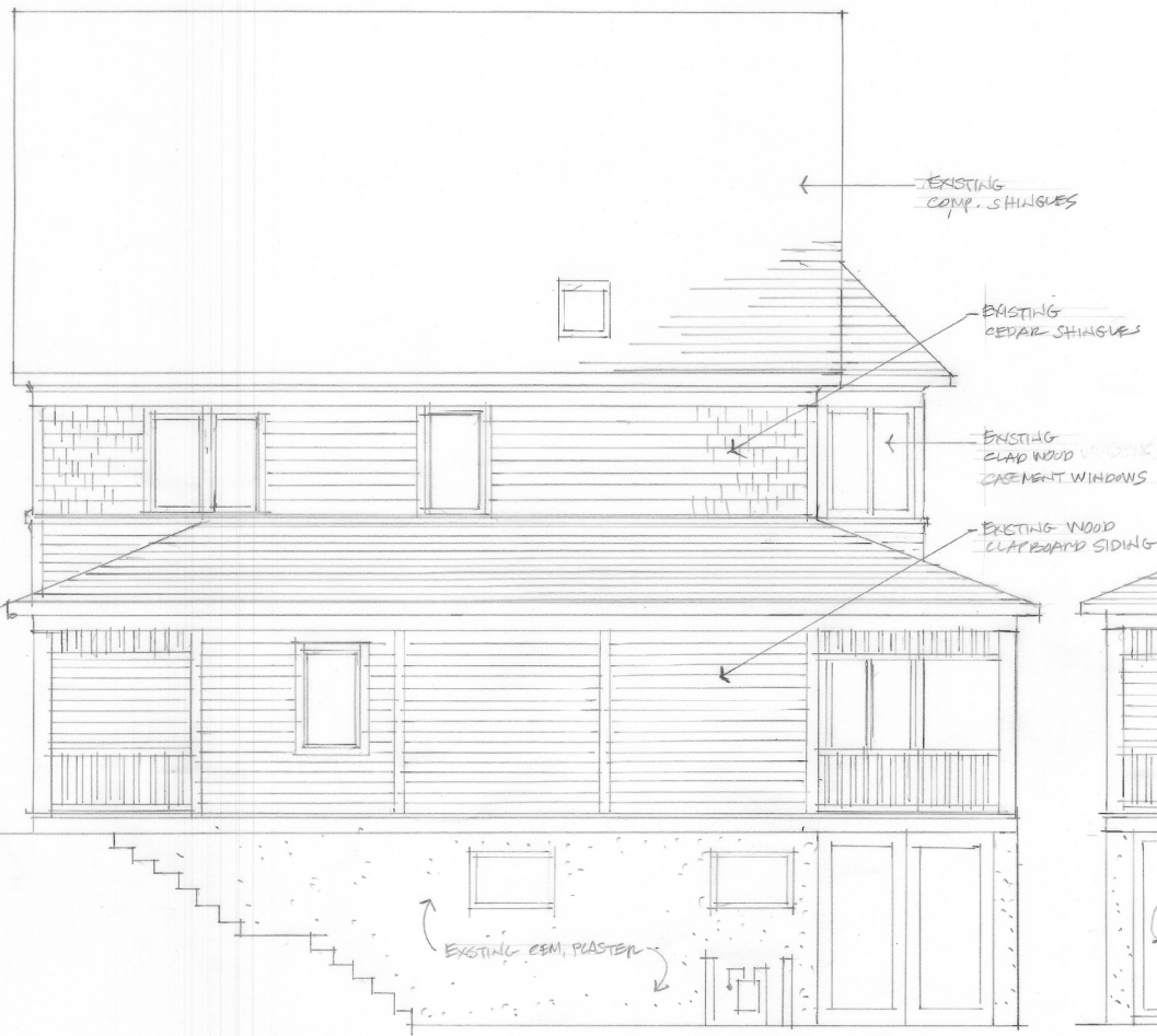
EXISTING SIDE ELEVATION
