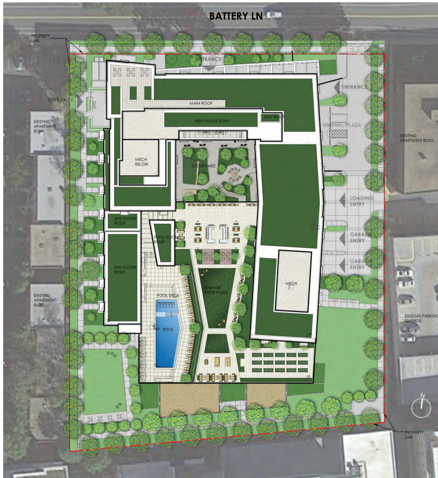
GREEN COVER WILL BE PROVIDED TO MEET OR EXCEED THE 35% REQUIREMENT BY UTILIZING A COMBINATION OF GREEN ROOF AREAS AND CANOPY COVERAGE AT THE GROUND LEVEL.
