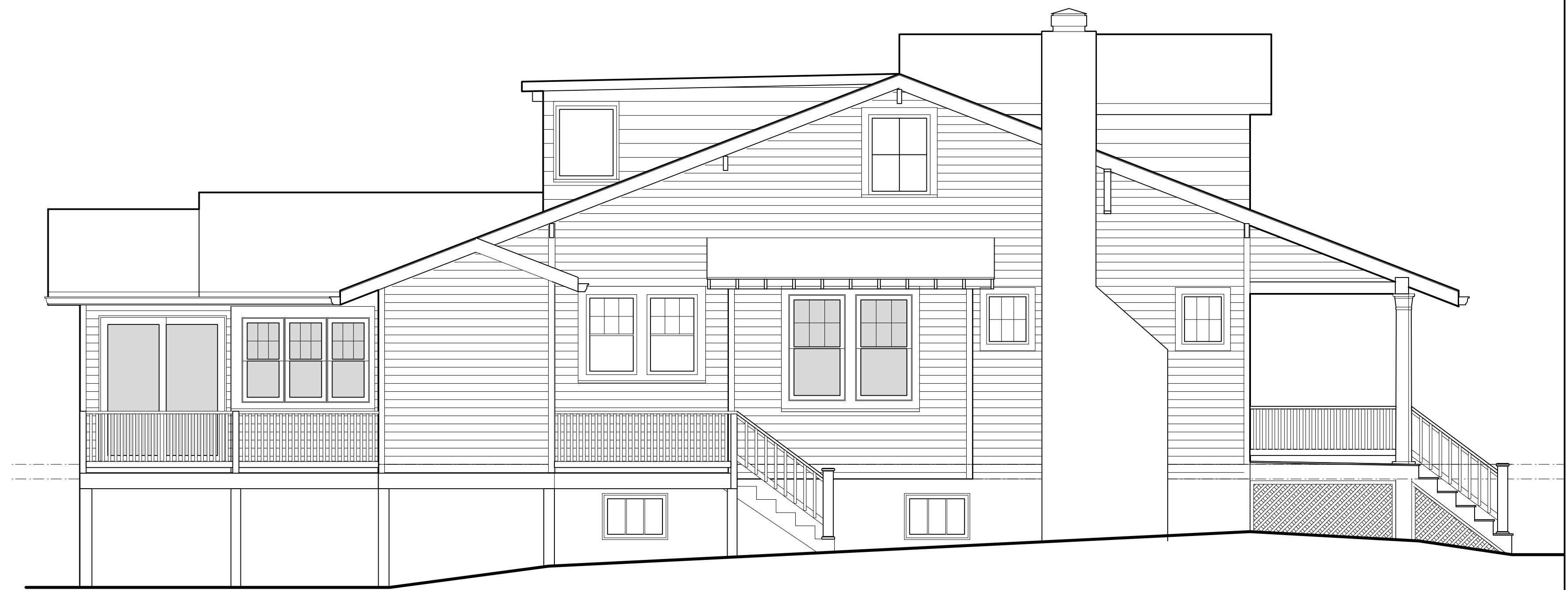
4 PROPOSED SIDE ELEVATION Scale: 1/4" = 1'-0"
