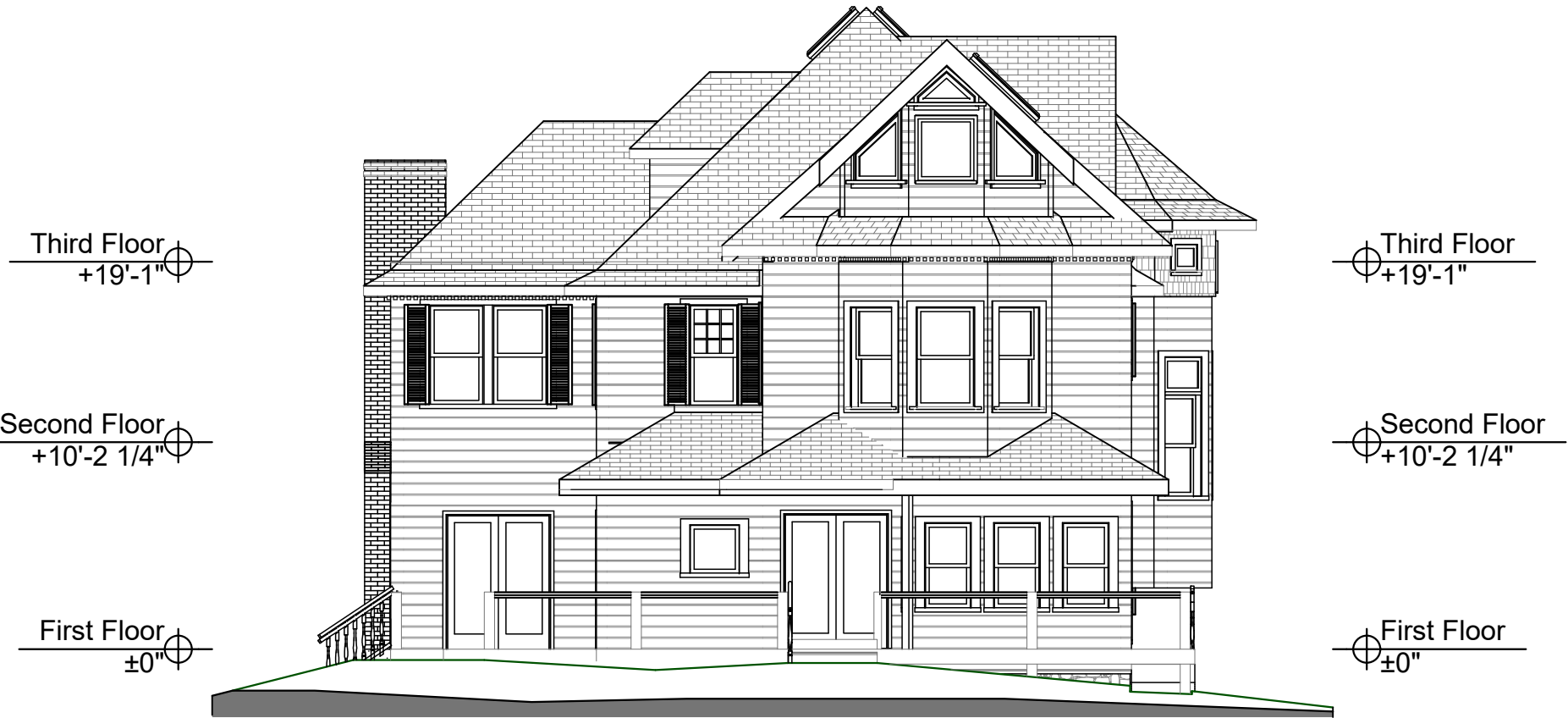
1 H.1.15 Rear Elevation-Existing SCALE: 1/8" = 1'-0"
