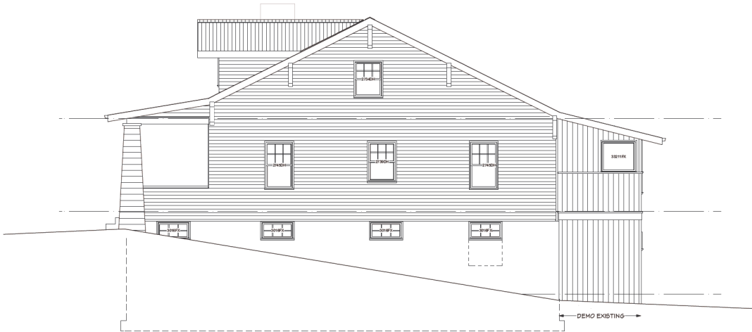
3 D002 WEST ELEVATION - DEMOLITION SCALE: 1/4" = 1'-0"
