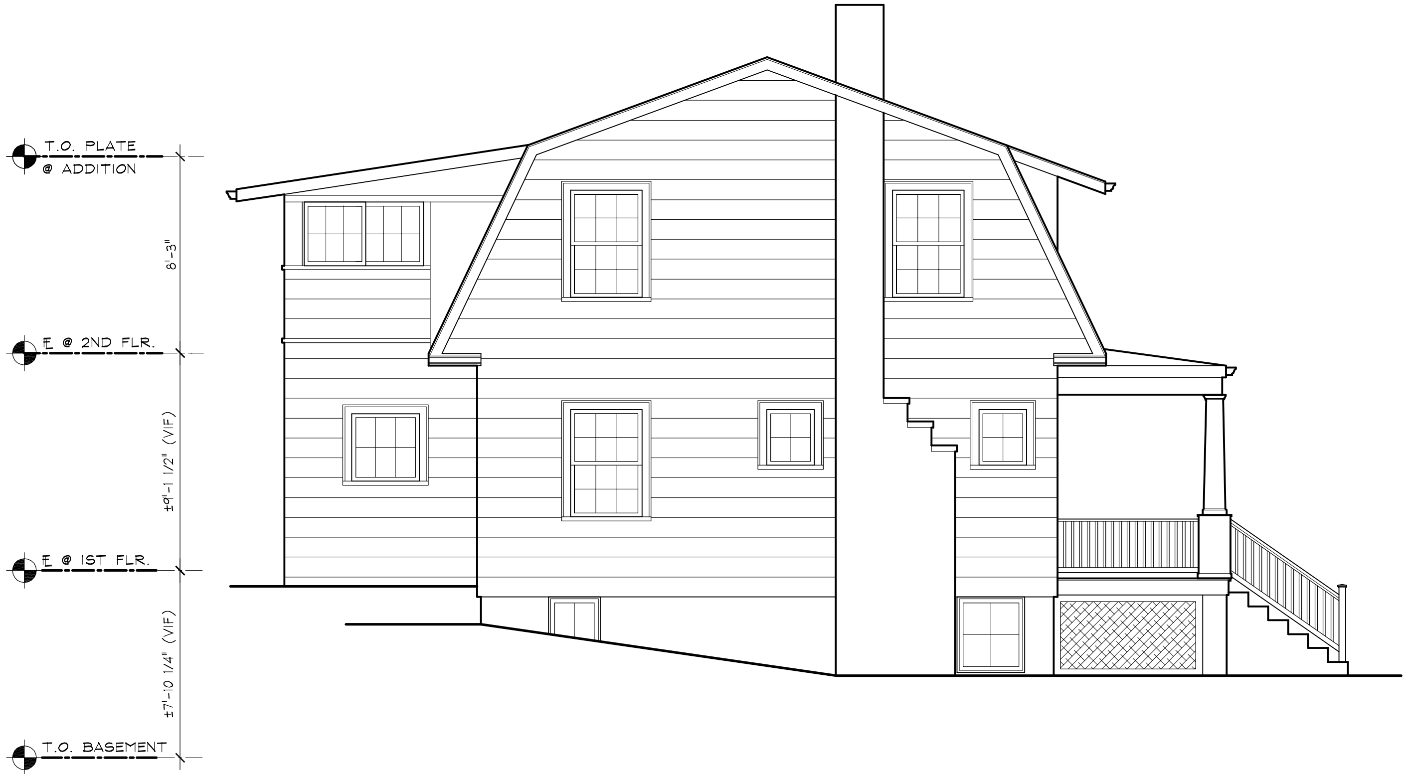
4 EXISTING SIDE ELEVATION A2.1 1/4" = 1'-0"
