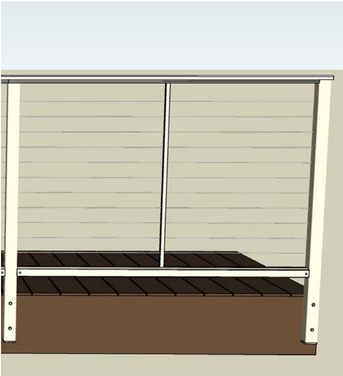
Figure 27: Example of non-compatible fascia-mounted railing system.
