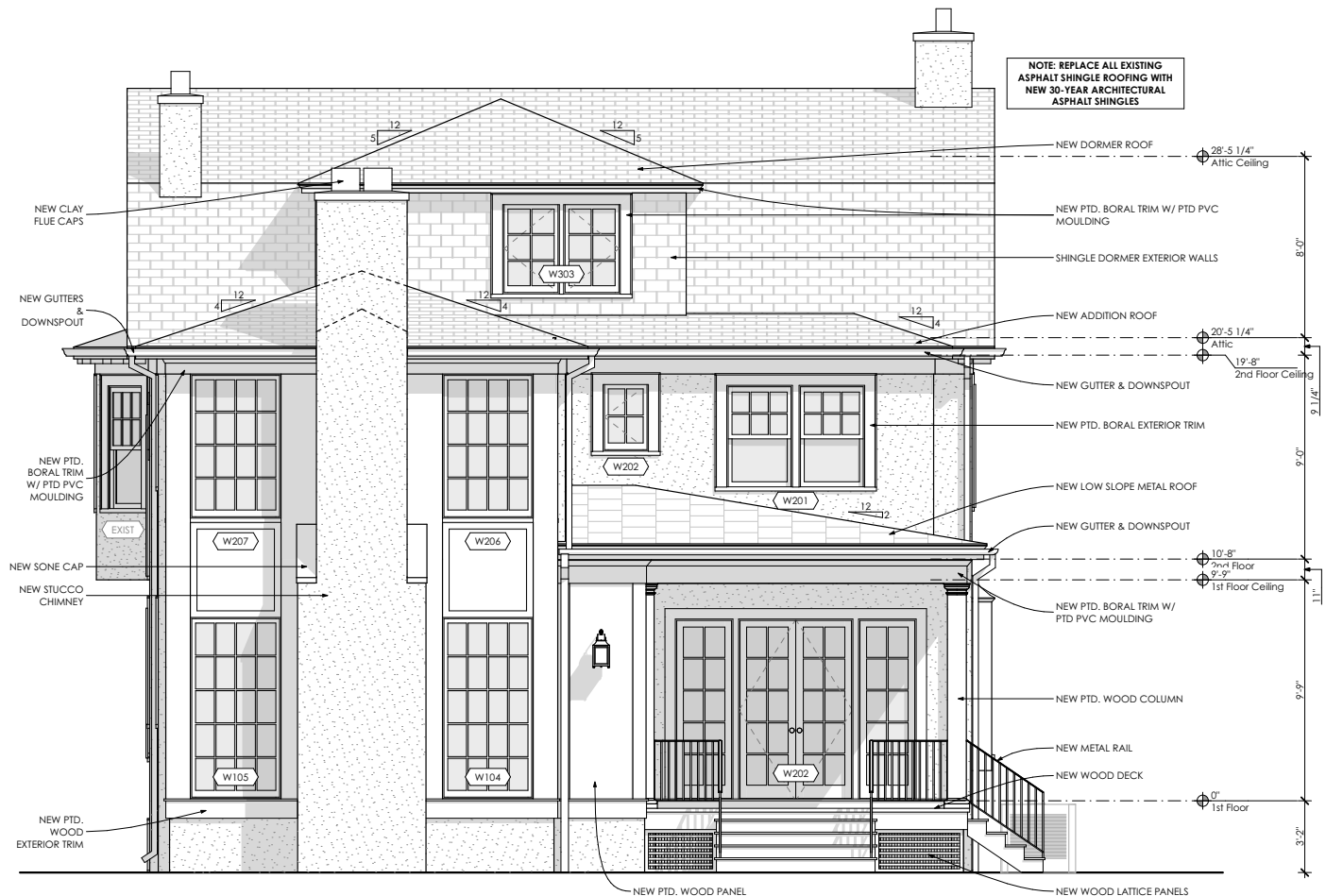
2 Proposed Rear Elevation 1/8" = 1'-0"
