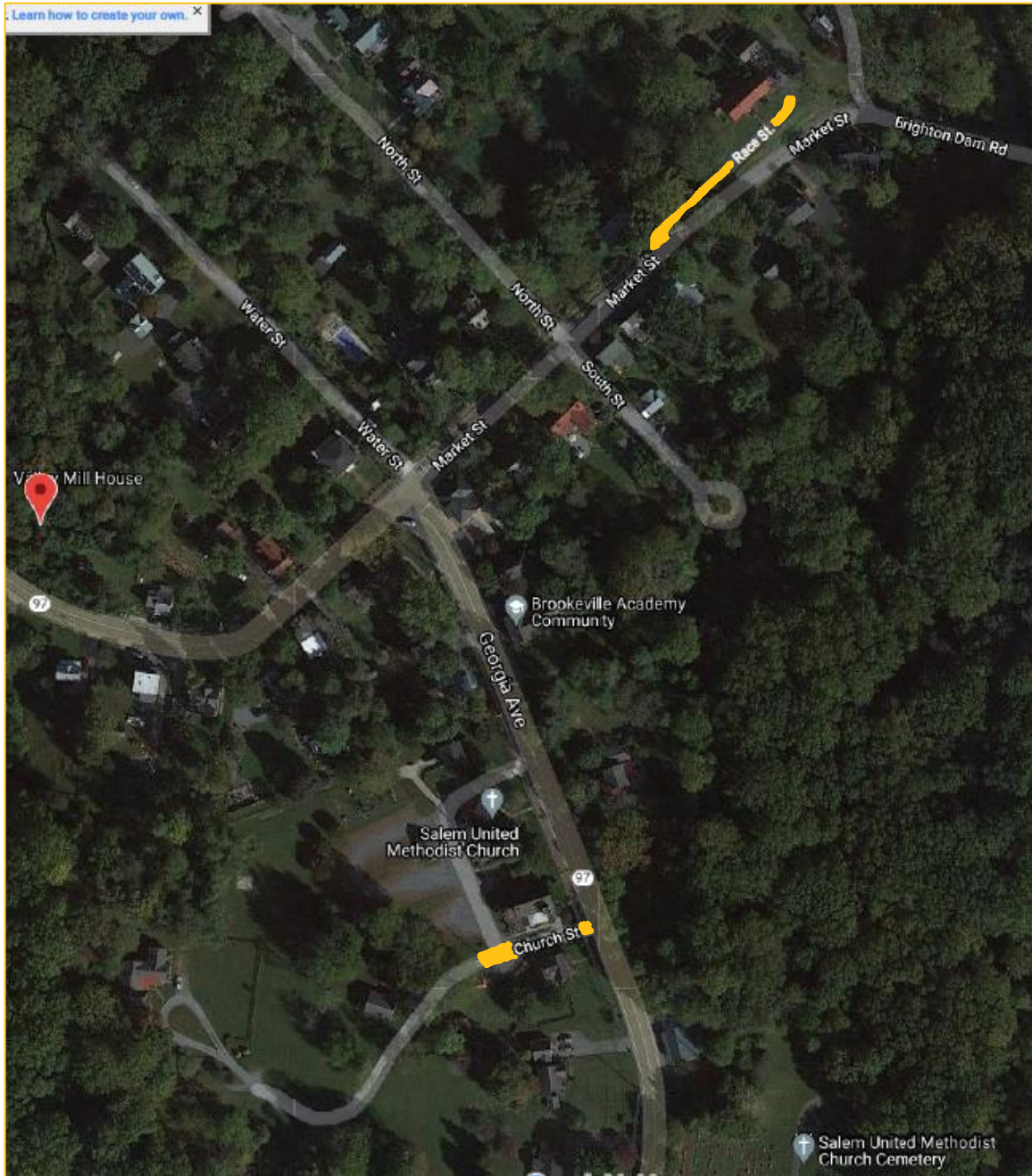
Figure A-3: Race/Church Street Tar and Chip Resurface (See Portions Highlighted in Yellow for Locations of Proposed Tar and Chip Surface)
