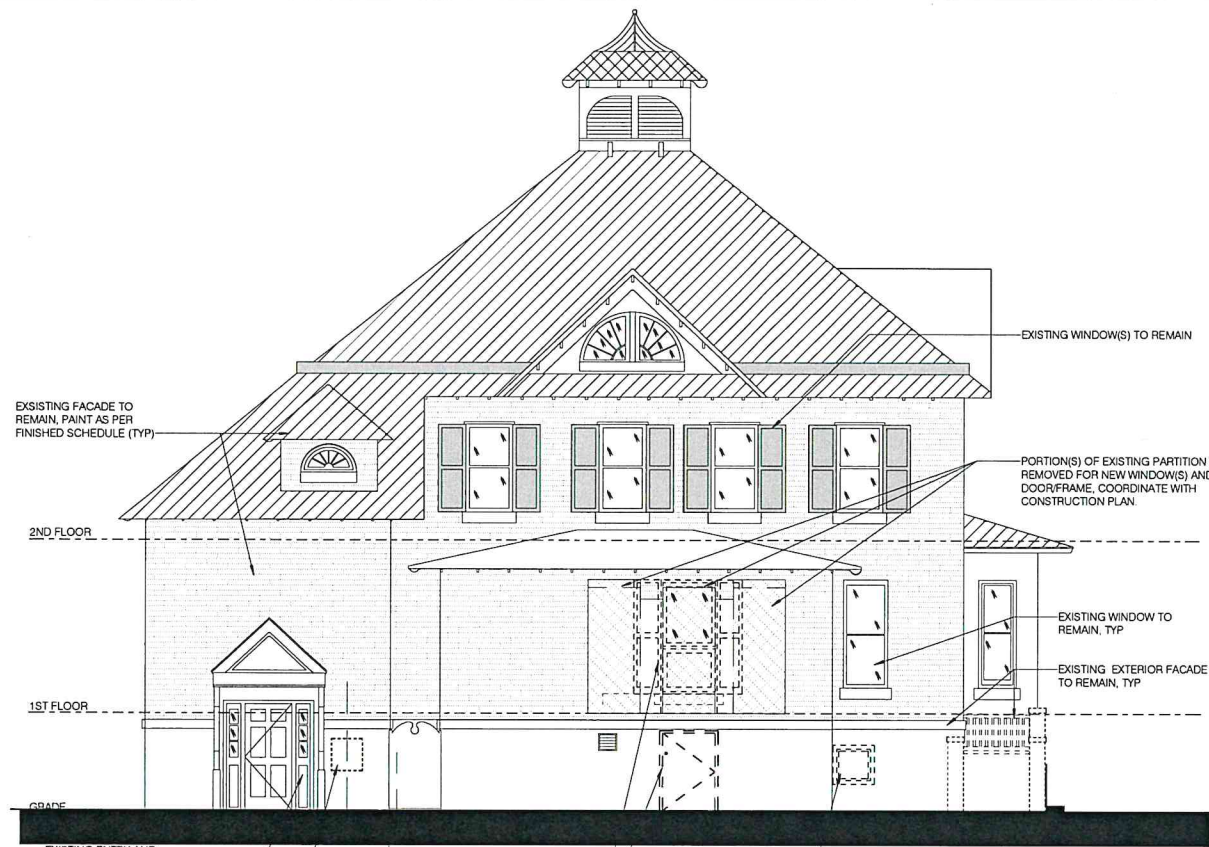
1 REMOVALS SCOPE AT SOUTH ELEVATION 3/16" = 1'-0"
