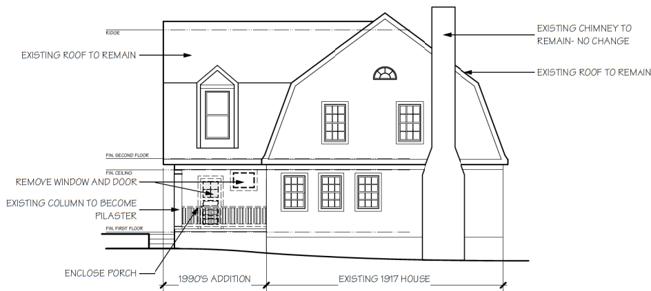
Existing/Demo Left Side Exterior Elevation Scale: 1/8" = 1'-0"
