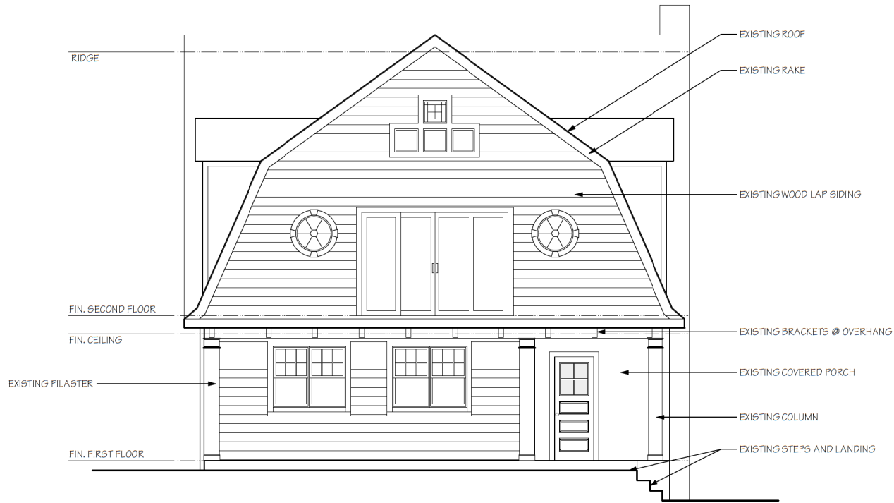
Existing Rear Exterior Elevation-1990's Addition Scale: 1/4" = 1'-0"
