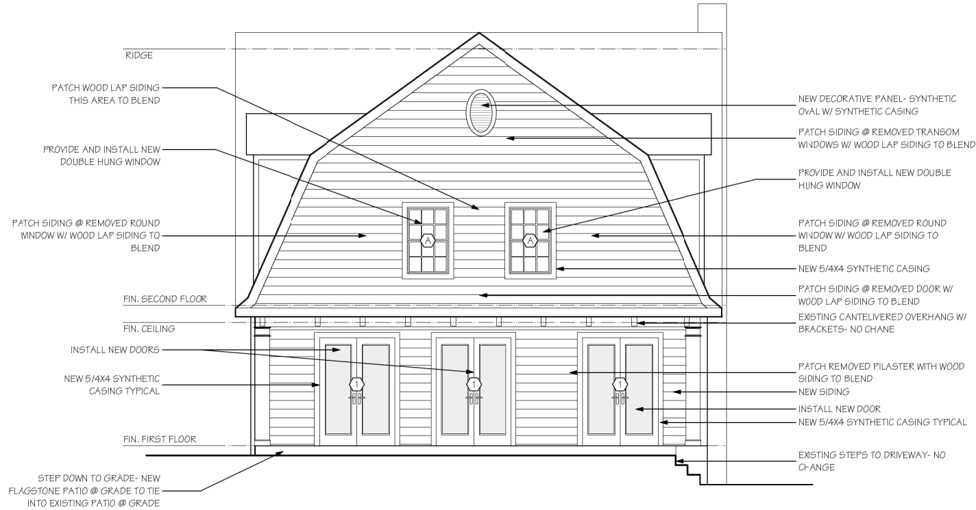
Proposed Rear Exterior Elevation Scale: 1/4" = 1'-0"
