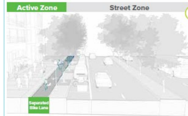
Figure 2-8. Separated Bike Lane
