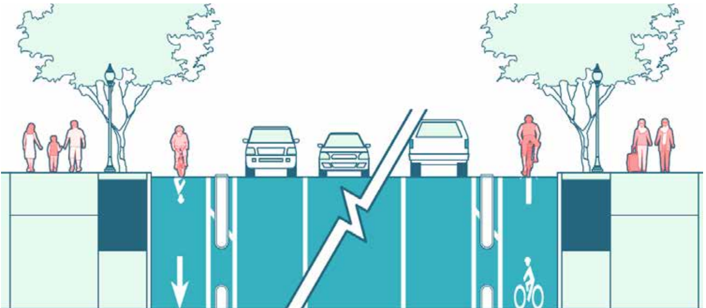
Figure 5-7. One-way Separated Bike Lane, Parking Separated, Interim Condition: Downtown Street, Town Center Street, Industrial Street
