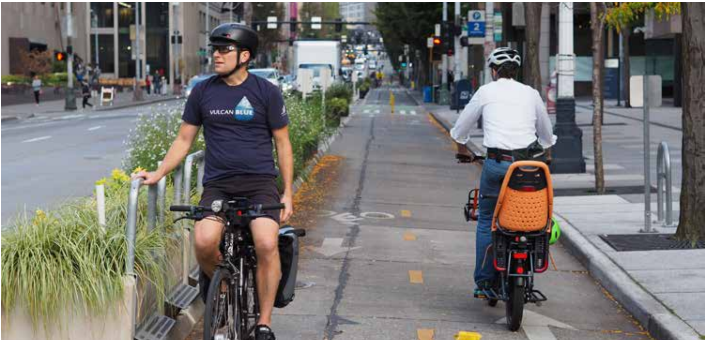
Figure 5-24. Example of bicycle lean rails and foot rests
