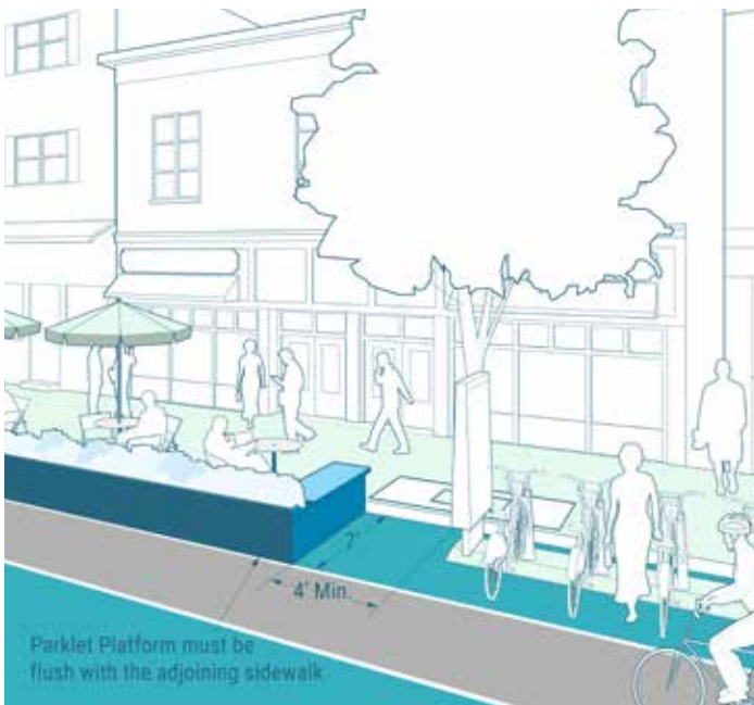
Figure 4-10. Illustration of parklet dimensions
