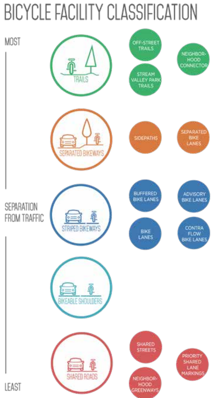
Figure 5-1. Montgomery County bikeway facility types (Source: Montgomery County Bicycle Master Plan)
