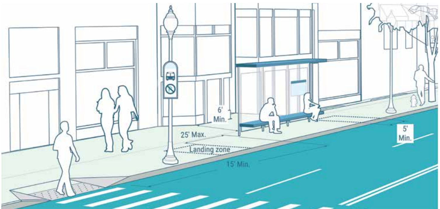
Figure 3-19. Illustration of bus shelter clearances
