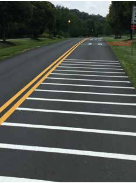
Figure 8-11. Example of optical speed bars
