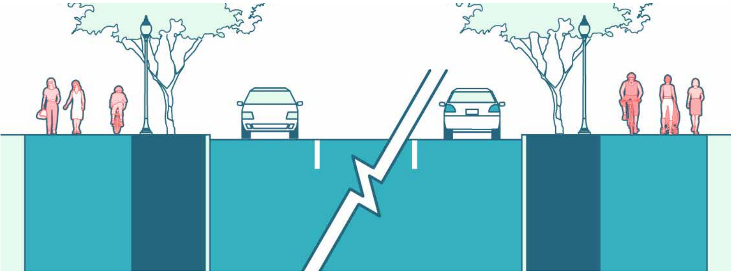
Figure 5-13. Sidepath, Both Sides, 6-8' street buffer: Boulevard
