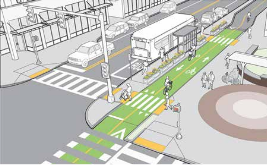
Figure 6-25. Floating bus island (Note: This graphic shows an intermediate-level bikeway, which is the county's default. This creates a detectable edge between the sidewalk and the bikeway.)
