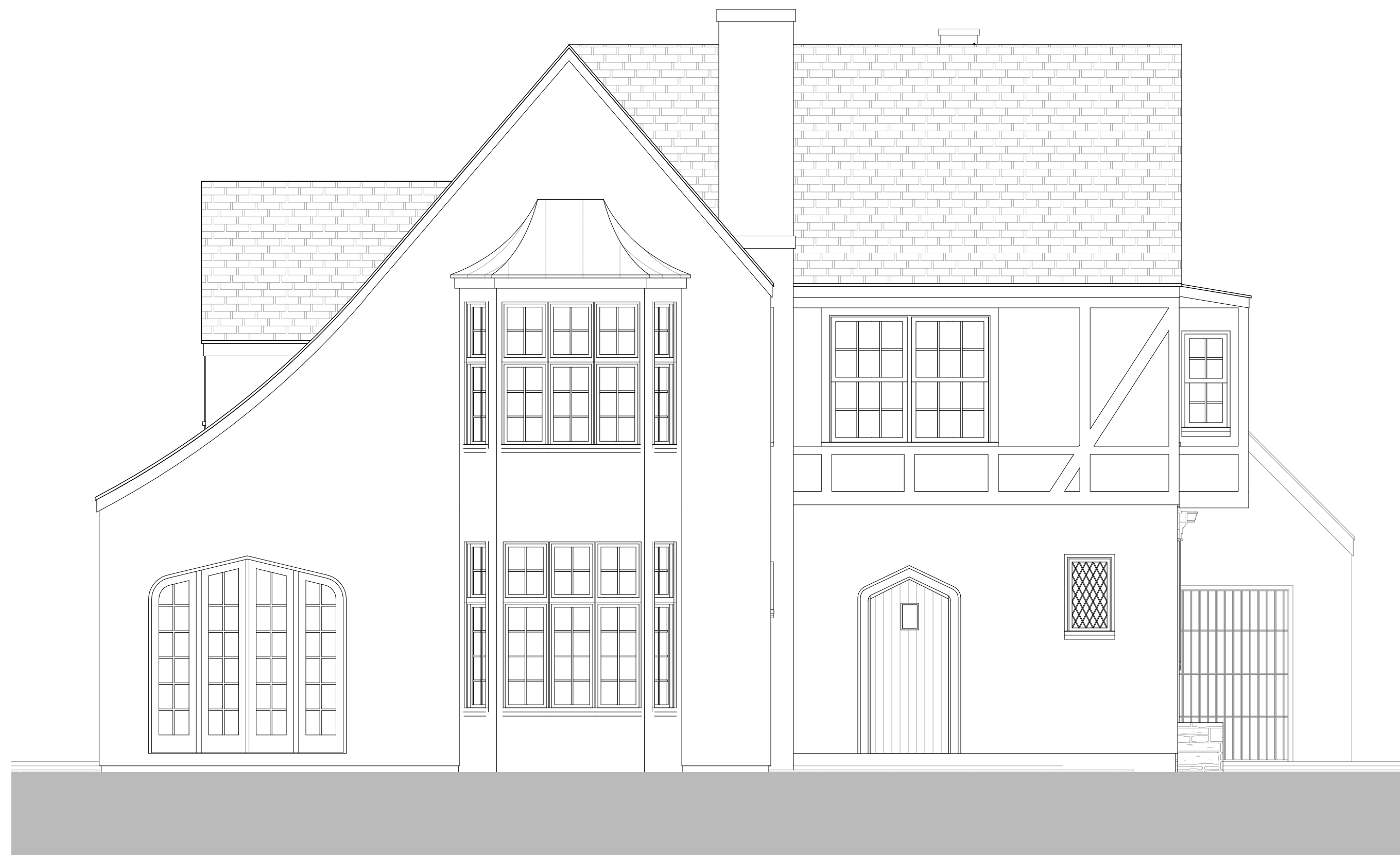
1 SOUTH ELEVATION OPTION 3 SCALE: 1/4" = 1'-0"
