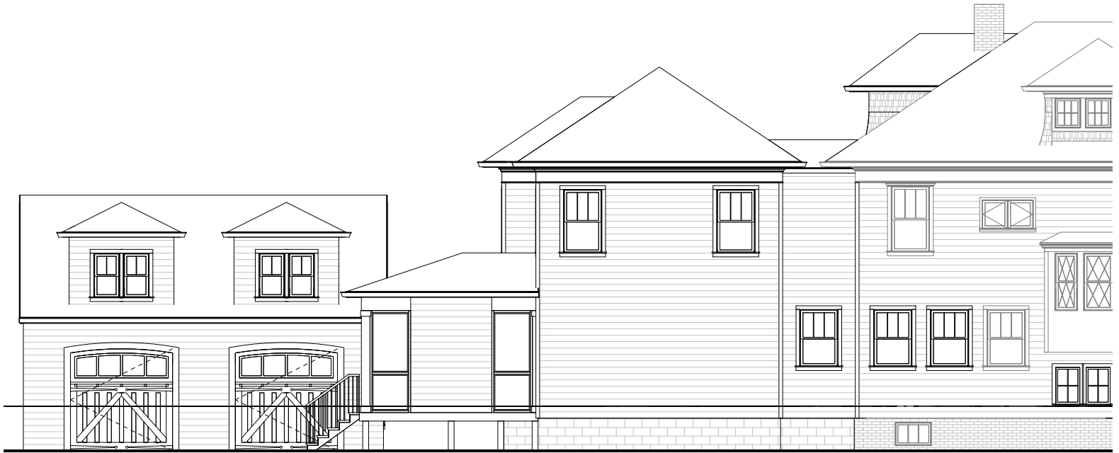
② Proposed Left Elevation w/ Garage 3/32" = 1'-0"
