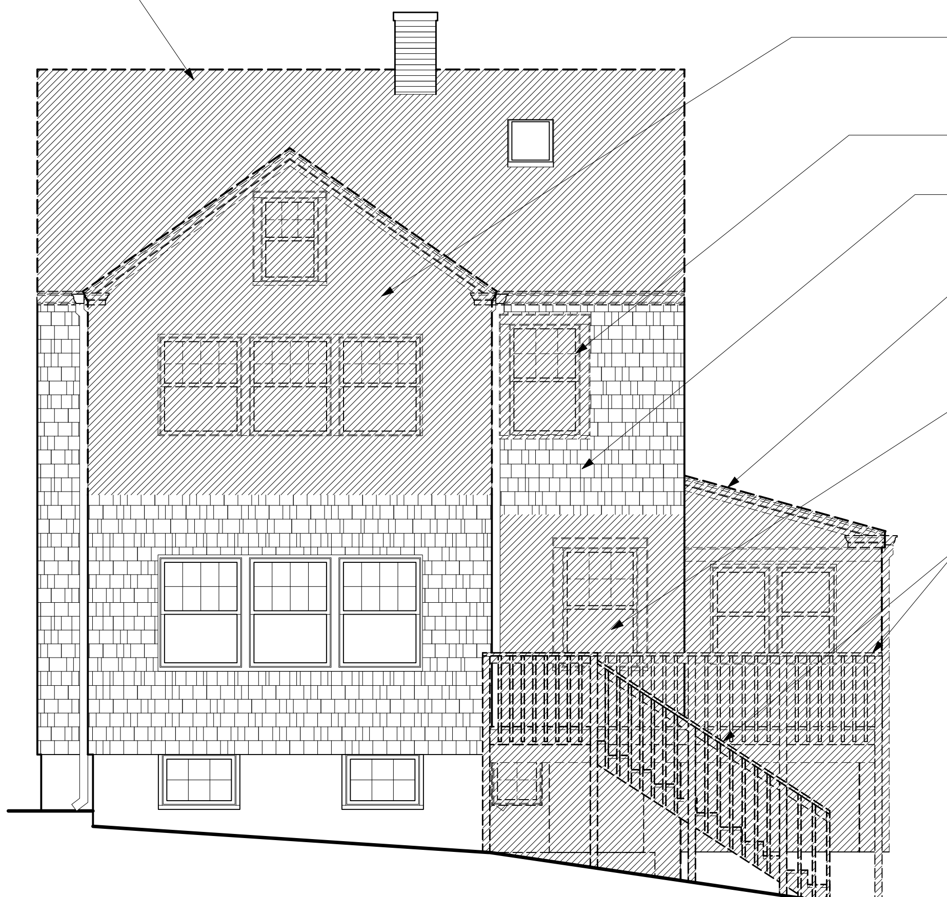
3 REAR / SOUTH DEMOLITION ELEVATION Scale: 1/4" = 1'-0"
