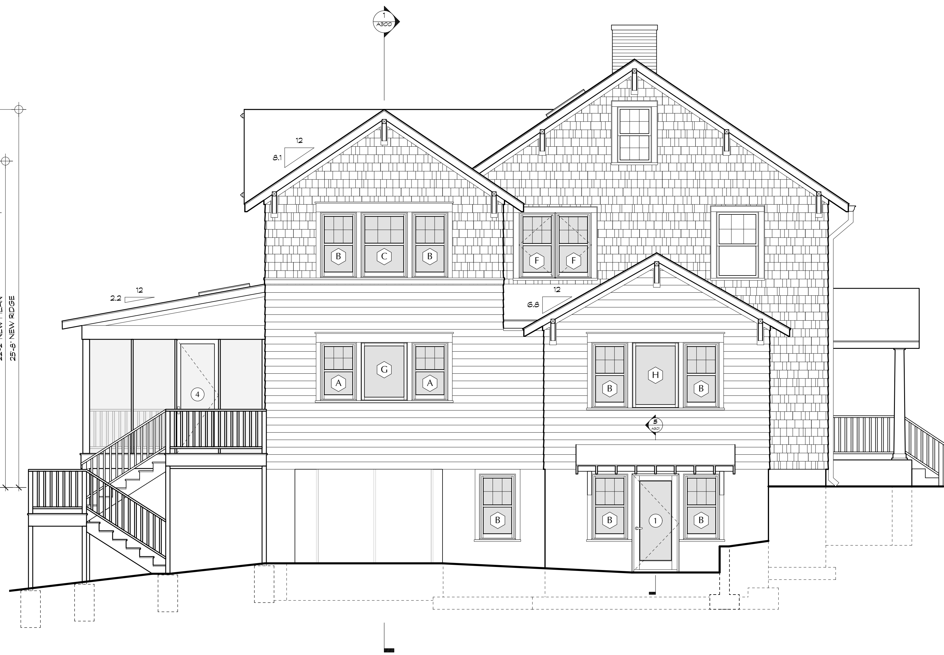
2 PROPOSED SIDE / EAST ELEVATION Scale: 1/4" = 1'-0"
