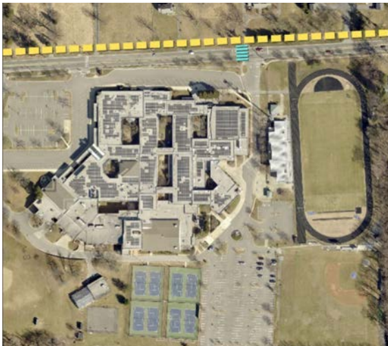
Figure 6. The recommended shared-use path is shown in yellow along the north side of MD 108. A new crosswalk and walk signal are recommended at the existing traffic signal at the high school's eastern entrance.
