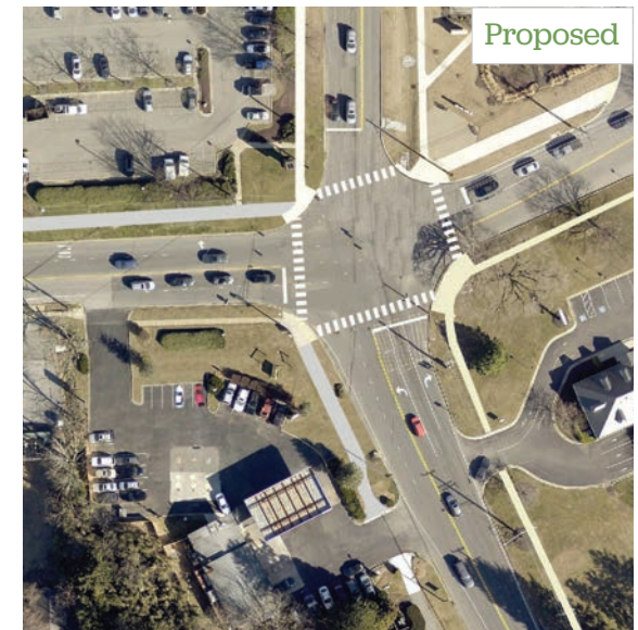
Figure 5. Revised intersection at MD 108 and MD 650 with marked crosswalks, new sidepaths and sidewalks, an increased turning radius in the northeast corner, and fewer driveways at the filling station in the southeast corner
