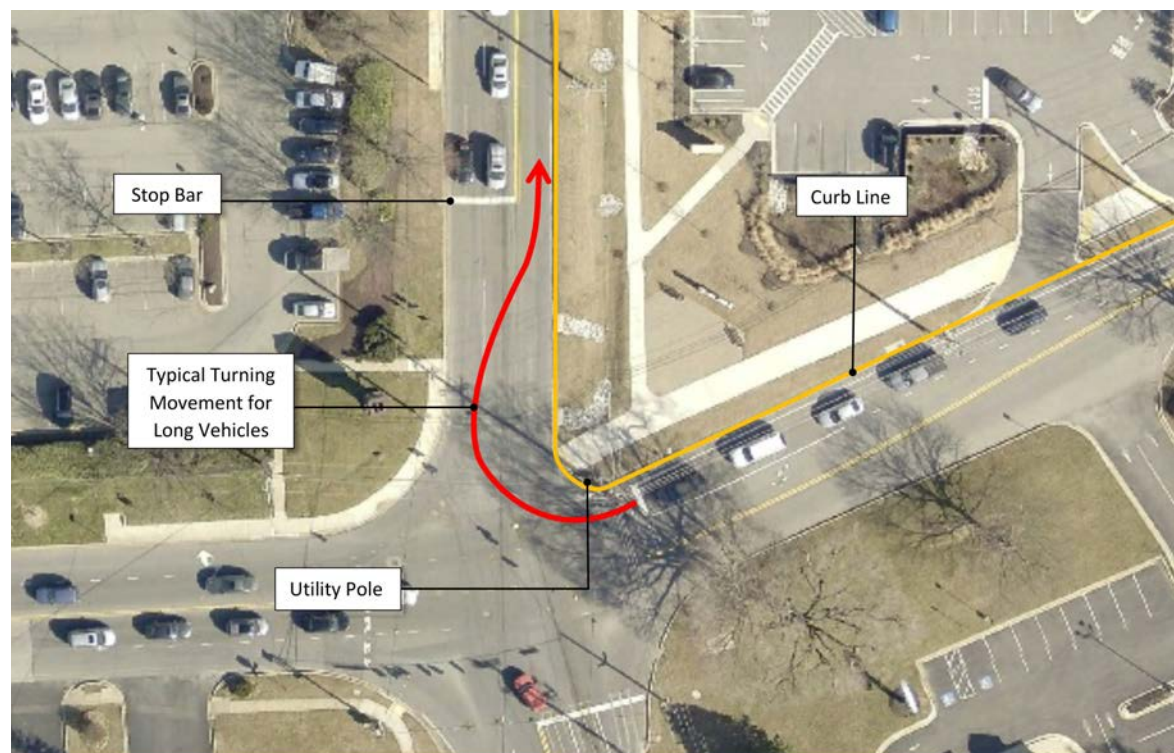
Figure 9. 2019 aerial view of the MD 108/650 intersection. The turning radius in the northeast corner is very tight, especially for longer vehicles and those with trailers, which led SHA to move the stop bar for southbound MD 650 well back from the intersection.
