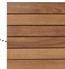
CUMARU WOOD TO BE USED FOR DECK FLOOR, RAILING, DECK APRON, AND DECK SKIRTING
