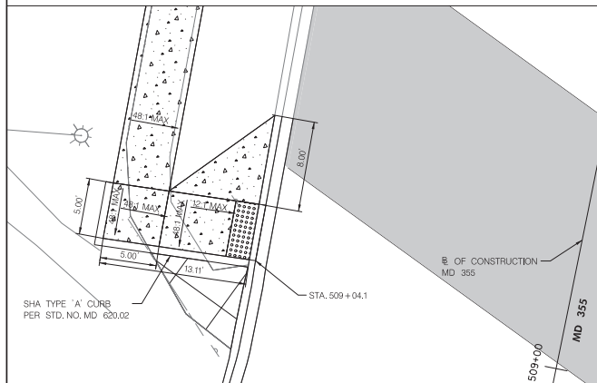
DETAIL C: SIDEWALK RAMP MD 355 MD 355 STA. 509+03.4 TO STA. 509+17.1
