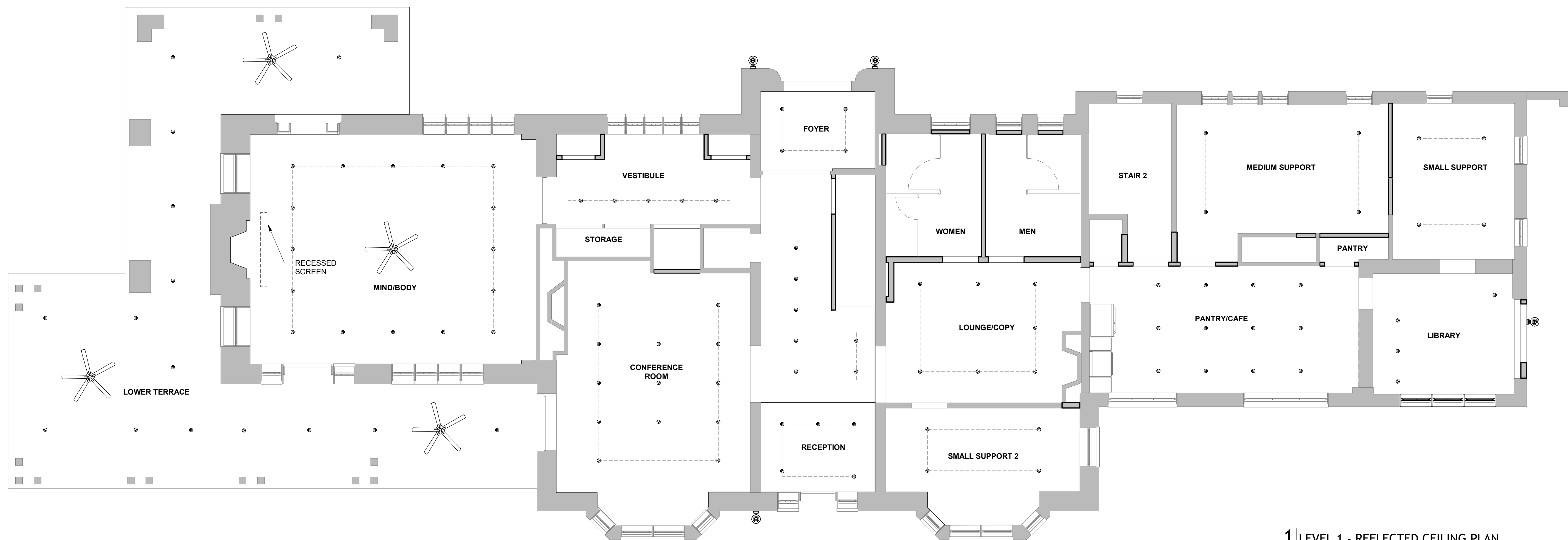
1 LEVEL 1 - REFLECTED CEILING PLAN A202 3/16" = 1'-0"
