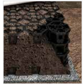
STRUCTURAL CELL DIAGRAM [GREEN BLUE URBAN, STRATA CELL]
