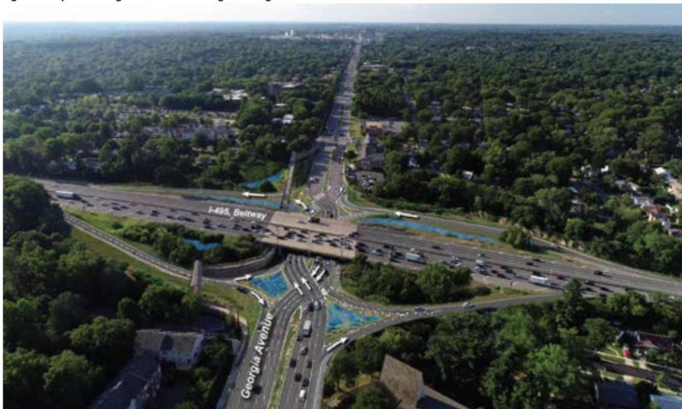
Figure 4: Proposed Diverge Diamond Interchange at Georgia Avenue and I-495
