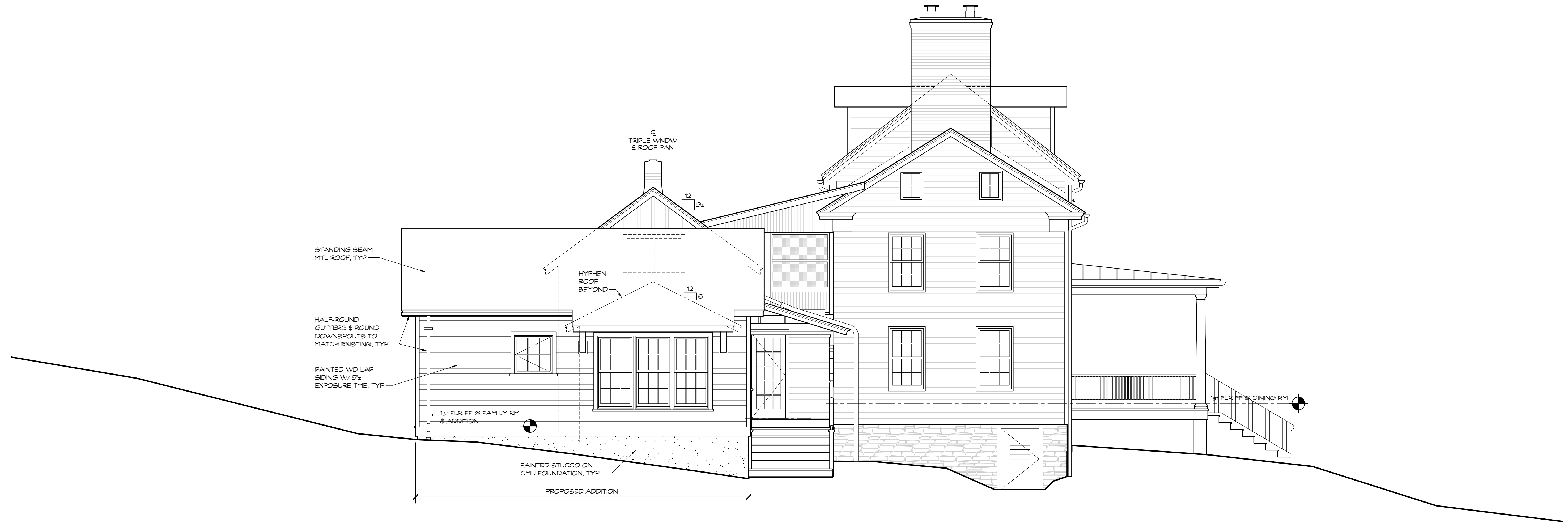
2 PROPOSED WEST (LEFT SIDE) ELEVATION A3.2 SCALE: 1/4" = 1'-0"
